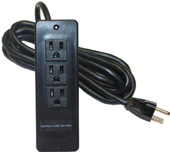
The three inline outlets power bar model **SF-PB3** accepts standard power cords with a 3rd outlet for oversized plug-in/transformer to accommodate cell phones and PDAs. It includes three grounded outlets. It has a 12 AMP rating and a 10 ft. 14-3 gauge power cord. The unit mounts in a 5-1/4" x 1-7/8" cutout. (Same cutout as PC-PATCH)
